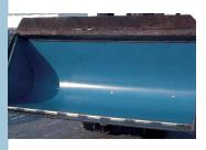
OKUSLIDE is also suited for the lining of wheel loader buckets, chutes and bunkers.
