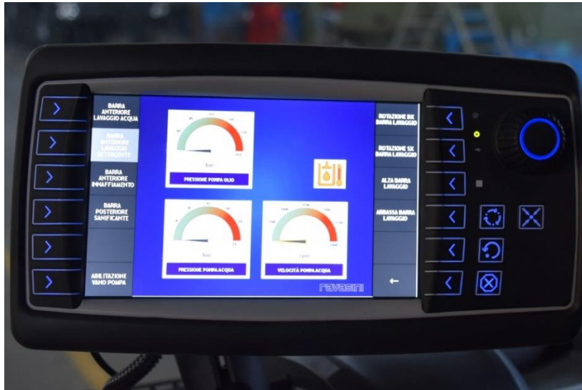
Digital display installed in the driver's cab
