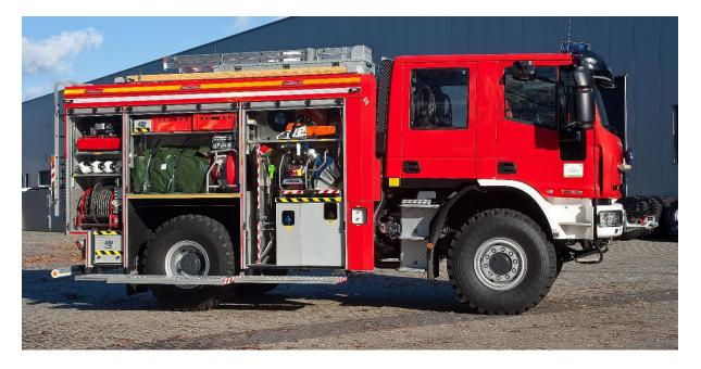
Above rear axle is located step integrated with fender construction allowing to take down equipment located inside locker
