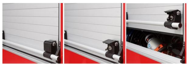
A total of 7 roller shutters are provided: 3 on each side of the vehicle and 1 at the rear of the vehicle, at the pump compartment. All materials and equipment are fixed in such a way that damage or blocking of the roller shutters is avoided. Automatic locker illumination is actuated by the roller shutters and/or foot boards and is controlled by a master switch with pilot light in the cabin.
