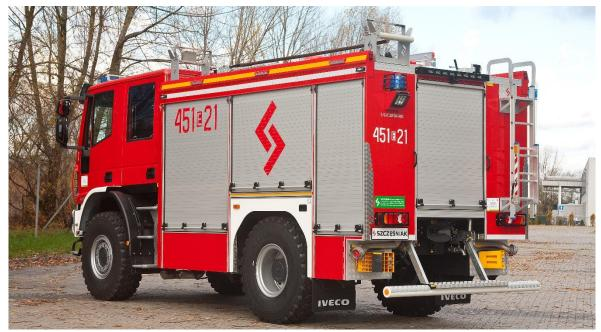
Place for extension ladder and the suction hoses are stowed on the roof, a stable ladder with non-slip steps is fitted at the rear of the vehicle for easy roof access. The necessary protection plates and hand rails are provided. All equipment in superstructure are securely fastened by means of rattle-free fixings. Heavier equipment is fixed on telescopic runners or on sliding frames.
