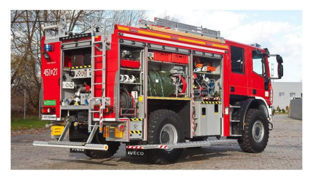
The water tank and the foam tank are fitted between the auxiliary equipment compartment, located behind the crew cab, and the pump compartment at the rear of the vehicle. Necessary draining vents for the leaking water are provided. The roof is covered with aluminum chequered non-slippery plates and is bordered by a gallery.
