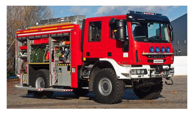
The bodywork of the vehicle is made of aluminum profiles and anti-corrosion treated hotgalvanized steel or aluminum panels. Critical areas are in closed steel tubing. The steel profiles have been treated internally against rust by means of a special injection wax. The whole body has been treated and professionally painted to give the vehicle a high resistance against rust. Underneath the vehicle an undercoat has been sprayed.
