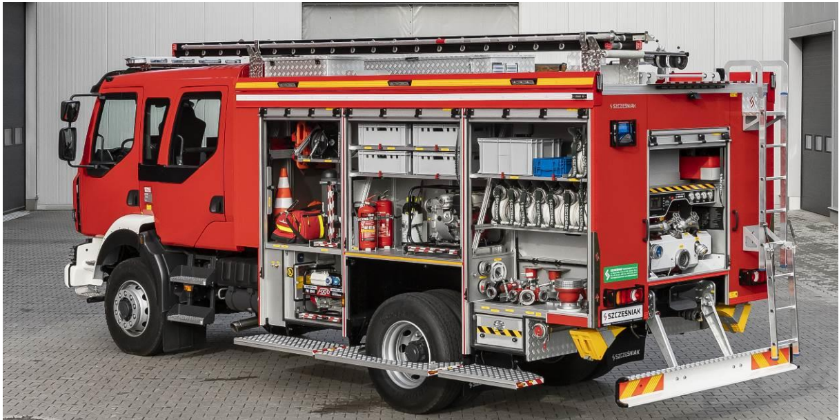
Example arrangement of equipment in the superstructure:
