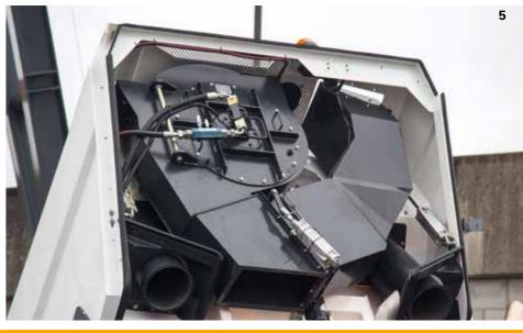
**5. Exhaust air management** Exhaust air can be directed rearwards from undernear or forwards from above, allowing drivers to respond to
