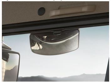
Electrically heated and adjustable rear view mirror, heated (392CZ) wide-angle mirror
