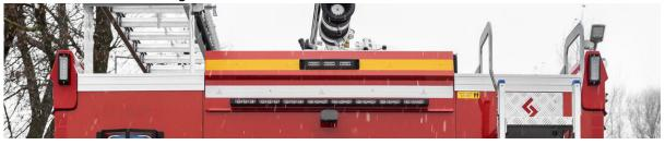
5. The vehicle is equipped with additional reverse gear lighting on the rear wall and under the cabin steps.
