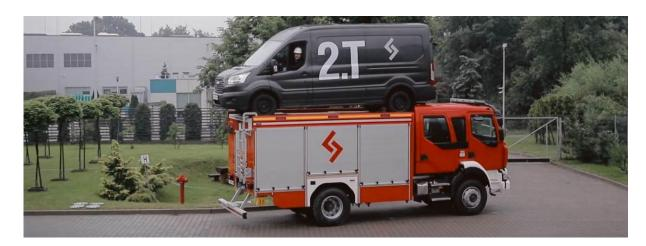
The roof of the building is made in the form of a working platform. Finished with anti-slip checker plate. The roof structure is adapted for the work of two firefighters. The designated communication path on the roof of the vehicle is flat and guarantees safe movement even after dark thanks to built-in lighting.
