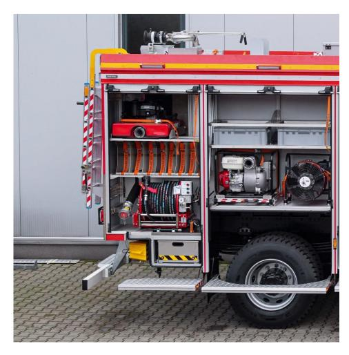
**Roof monitor:** In the rear roof part there is a manually controlled water and foam roof cannon with adjustable capacity from 800 l/min. up to 2,400 l/min. and a throw range of 60 m. The gun is equipped with a pressure gauge and a pressure cut-off valve.
