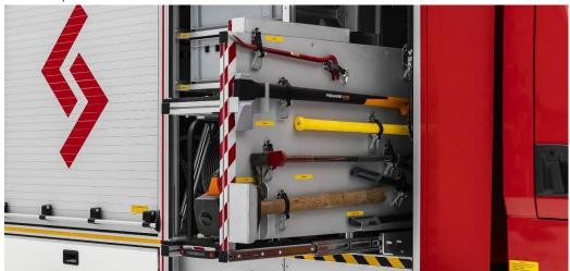
Each drawer has ergonomic handles, the hydraulic drawer allows you to assemble the entire set in one place. The drawer system allows, after some time of use, to be modified for a new set without any significant modifications:
