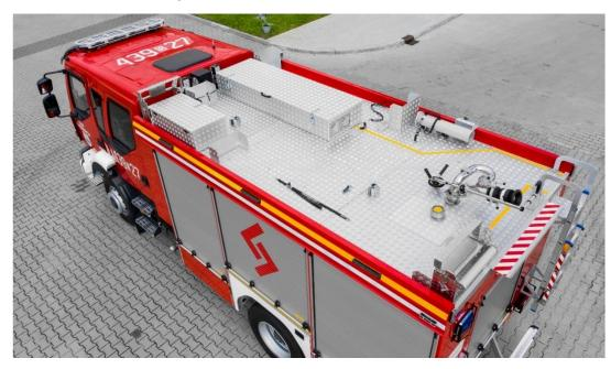
A solid ladder to access the roof, mounted on the rear wall. Additional handrails at the top of the ladder to facilitate climbing and an additional full step at the top. The ladder rungs are anti-slip.
