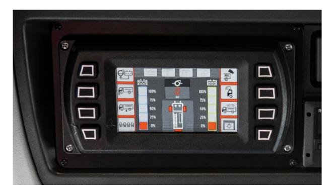
Control panel In The car pump compartment is based on a 7-inch display equipped with 10 buttons and enabling control of:
