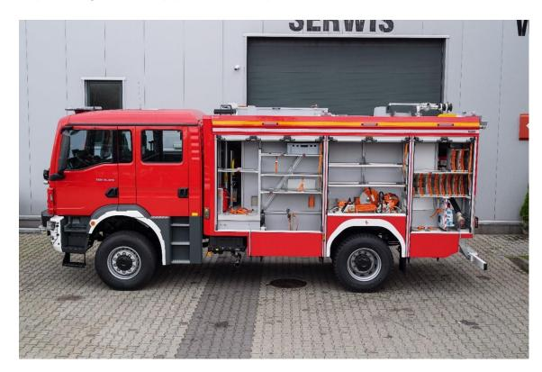
In the front part of the structure there is space for long elements that are often used during operations. There is a mount for medical equipment such as a stretcher, Kramer splints or a medical bag. The front compartment has a retractable panel with a mount for two Breahing Apparatus cameras and a drawer with a power generator.
